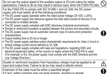
Do not use the output signal of the auxiliary output or IO-Link output for safety
