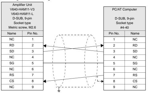
Ground shielded wires either at the CIDRW Controller side or at the PC/AT computer side.
