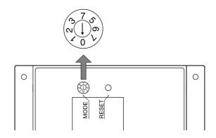
**3.** When all of the devices to be used are connected, turn the power ON. Start up in the Normal Operation mode.
