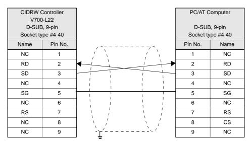
Ground shielded wires either at the CIDRW Controller side or at the PC/AT side.
