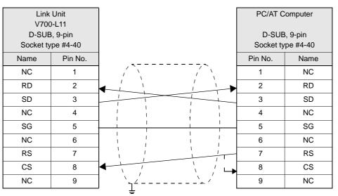
Ground shielded wires either at the CIDRW Controller side or at the PC/AT computer side.
