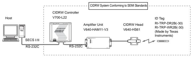
The V640-HS61 CIDRW Head can be connected to V640-HAM11-V3 Amplifier Units to communicate with ID Tags.
