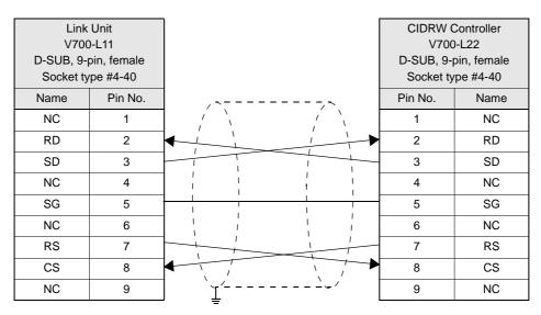
Ground shielded wires at the CIDRW Controller side.
