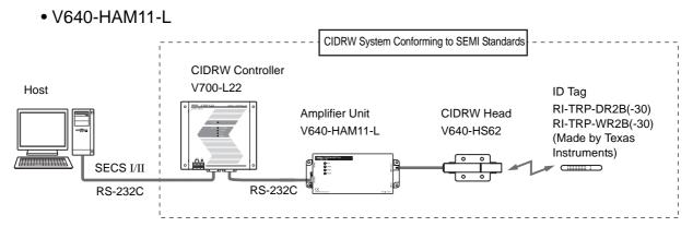
The V640-HS62 CIDRW Head can be connected to V640-HAM11-L Amplifier Units to communicate long-distance with ID Tags. The functions of the V640-HAM11-L Amplifier Unit are the same as the functions of the V640-HAM11-V3 Amplifier Unit.
