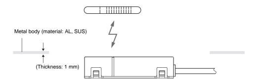
However, ensure the distances indicated below between the CIDRW Head and the metal body. If you do not ensure these distances the communications distance will be substantially shortened.
