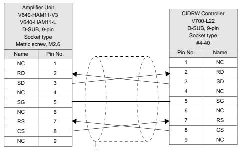
Ground shielded wires either at the Amplifier Unit side or at the CIDRW side.
