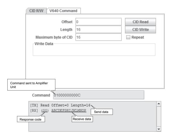
Only visible ASCII characters can be used to read and write data on the CID R/W Tab Page. If characters that are not visible ASCII characters are detected for a CID read, they will be converted to asterisks (\*).
