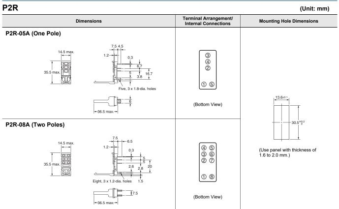
Note: If an I/O SSR or Indicator Module is used, the polarity of terminal 1 is negative.
