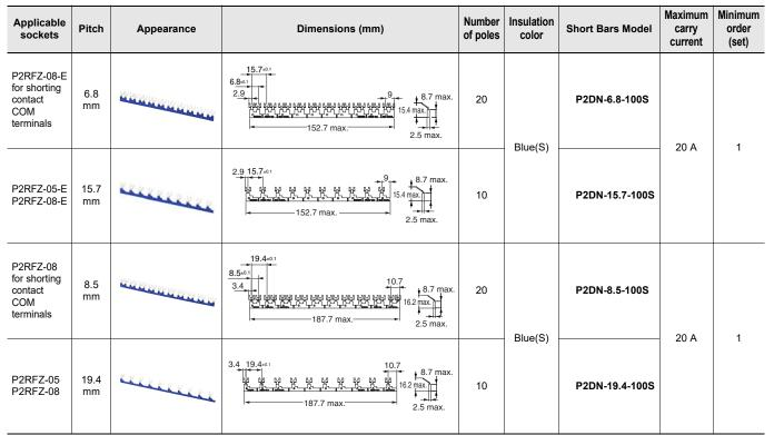
Note: 1. Select an applicable type of short bars by checking applicable socket type, appearance, and dimensions.
