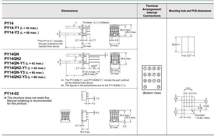
Note: 1. Use a panel with a thickness of 1 to 2 mm when mounting a Socket on it.
