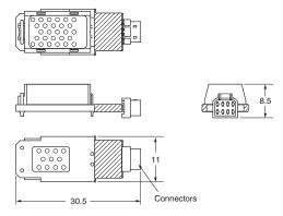
Note: Firmly insert the connector all the way in when mounting the ES2-M-N to the Sensor.
