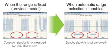
Note: If a measurement value becomes 5% or less than the rated current, the minute range is selected.
