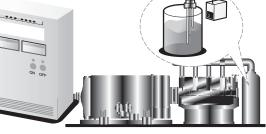
Cut costs by using the 61F in situations where ultrasonic/electrostatic capacity level controllers were used because only DC power supply was available.
