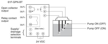
Note: 1. The part within the dotted-line box is for the 61F-GPN-BC (relay-output type) only.2. The power supply does not have any polarity.
