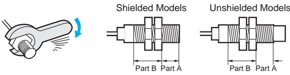
Note: 1. The allowable tightening strength depends on the distance from the edge of the head, as shown in the following table. (A is the distance from the edge of the head. B includes the nut on the head side. If the edge of the nut is in part A, the tightening torque for part A applies instead.)
