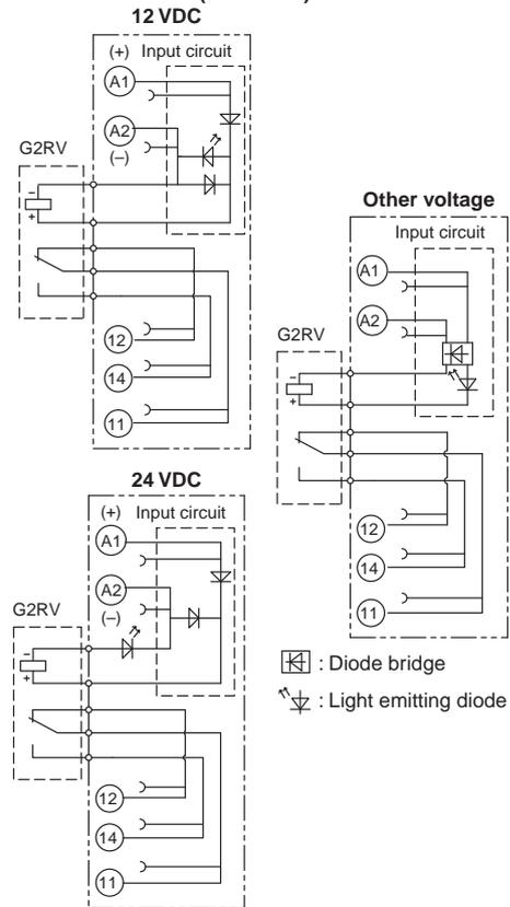
**Models with latching lever (with test switch)**
