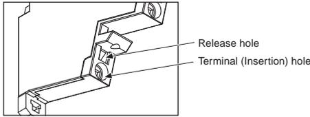
**Connecting Wires with Ferrules and Solid Wires**
