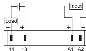
**Note:** The load can be connected to either the positive or negative terminals.
