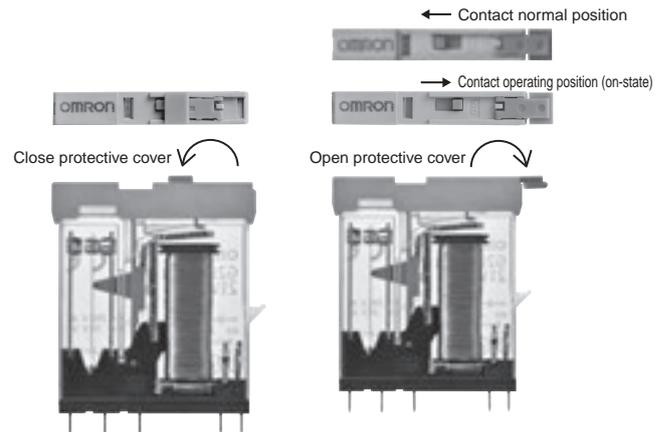
Keep the protective cover open when using the latching lever. Move until the latching lever clicks to the ON position (ON state). After use latching lever, in order to prevent malfunction, return the switch to contact normal position (OFF state), and make sure the protective cover is firmly closed.
