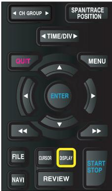
This key is used to switch the window mode.
