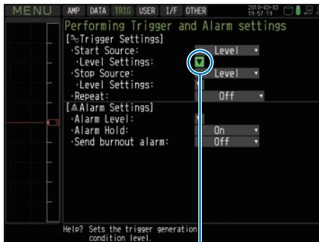
Place the cursor here and press the ENTER key to open the following setting screen.
