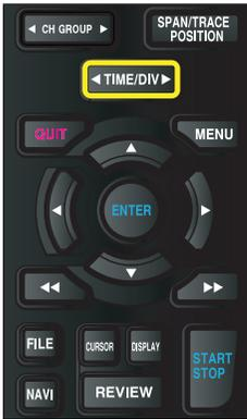
Press the left/right key of the TIME/DIV key to change the time axis display width.
