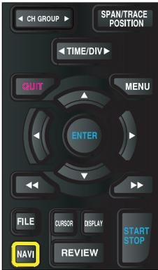
This key is used to display the key operation content during Free Running, capture or replay.
