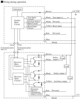
\*1 Emission is stopped : 1/2 Vs to Vs or open Normal operation : 0 V to 3 V.
