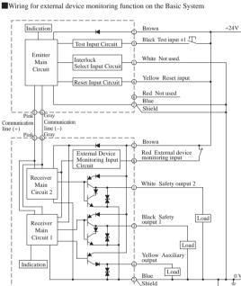
\*1 Emission is stopped : Short-circuited to Vs-3 V to Vs Normal operation : Short-circuited to 0 V to 1/2 Vs or open Wiring to disable external device monitoring function on the Short-circuit the external device monitoring input to the auxiliary
