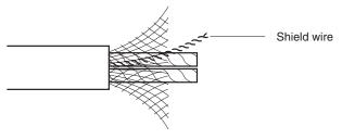
Remove the exposed mesh and the aluminum tape from the signal and power lines. Strip the covering from the signal and power lines to the proper length for the crimp terminals. Twist together the wires of each of the signal and power lines.
