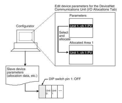
**Note** The maximum allocation size for the IN and OUT Areas (100 words) applies to the DeviceNet Communications Unit, and does not apply to the size of allocations in the Master Unit. For details on allocation sizes in the Master Unit, refer to the operation manual for the Master Unit being used.
