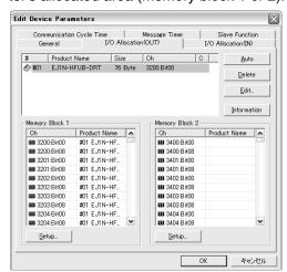
4. Click the Edit Button, and edit any of the I/O allocations. Set where to allocate the master's IN and OUT Areas in the Allocated field. When the master's IN and OUT Areas consist of two blocks, specify in which block to allocate the data.
