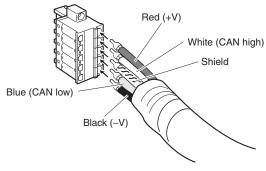
Colored stickers that match the colors of the lines to be inserted are provided on the Master Unit and slaves. Use these stickers to check that the lines are wired correctly. The colors correspond to the signal lines as follows:
