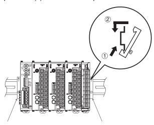
Note Always use two End Plates to clamp the Units together from both ends.
