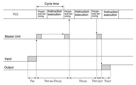
T<sub>IN</sub>: The Input Slave's ON (OFF) delay (Minimum value: 0)
