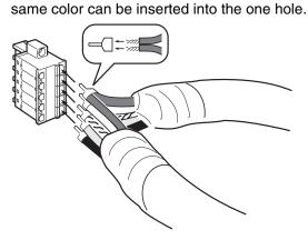
Crimp the two lines together that are to be inserted into the same hole using a special crimp terminal, as shown in the following diagram.
