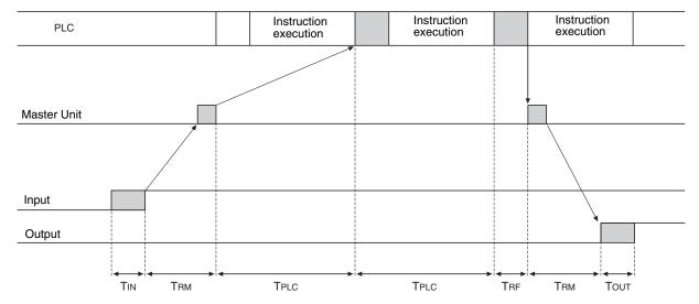
T<sub>IN</sub>: The Input Slave's ON (OFF) delay
