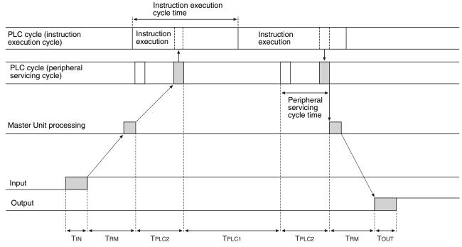
T<sub>IN</sub>: The Input Slave's ON (OFF) delay
