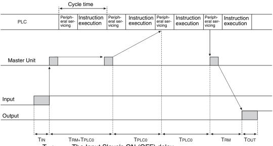
T<sub>IN</sub>: The Input Slave's ON (OFF) delay
