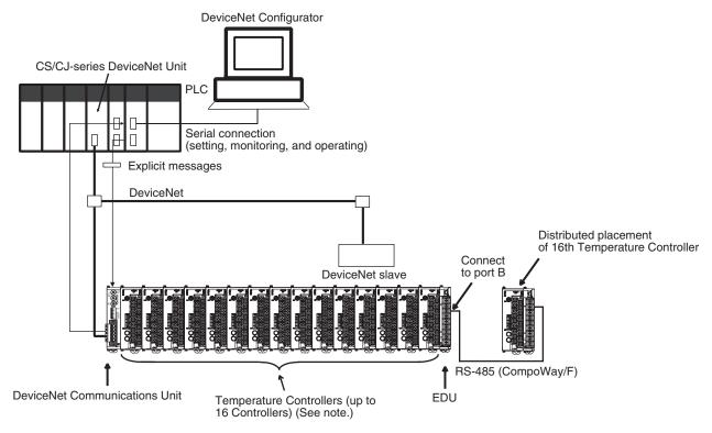
Note: Up to 16 Temperature Controllers can be connected to one DeviceNet Communications Unit. Use distributed placement via RS-485 for the 16th Temperature Controller.
