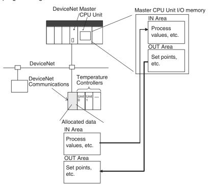
Use either of the following two methods to allocate DeviceNet Communications Unit I/O in the master.
