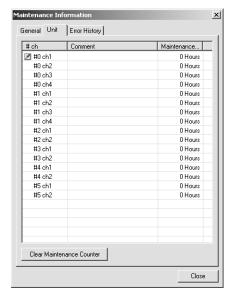
The following information can be confirmed for each of the Temperature Controllers connected to the DeviceNet Communications Unit.
