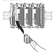
Using the Connector Provided with the DeviceNet Communications Unit for a Multidrop Connection (Using Thin Cables)
