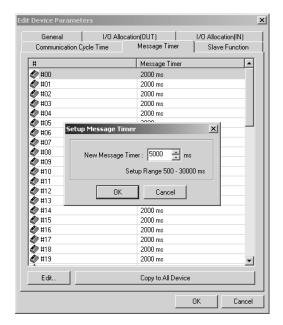
Click the **General** Tab in the Edit Device Parameters Window, and then click the **Download** Button. The parameters will be downloaded and the value for the message monitor timer of the DeviceNet Communications Unit will be changed.
