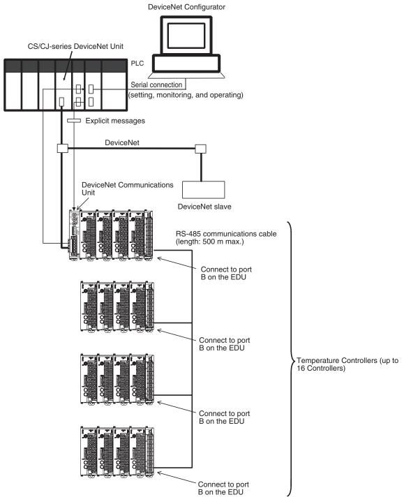
Connect the master and DeviceNet Communications Unit to port B (RS-485) of each End Unit.
