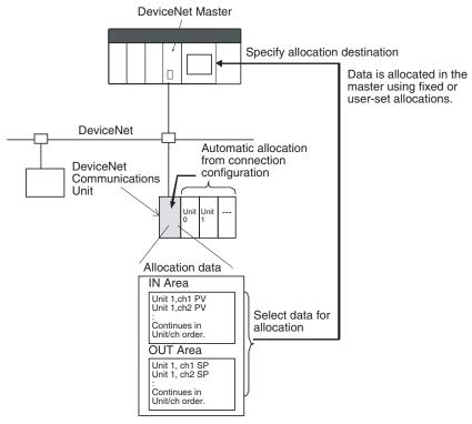
Note: The above allocation data is automatically allocated according to the connection configuration.
