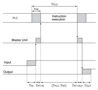
T<sub>IN</sub>: The Input Slave's ON (OFF) delay (Minimum value: 0)
