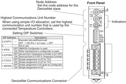
This connector connects the DeviceNet network communications cable.
