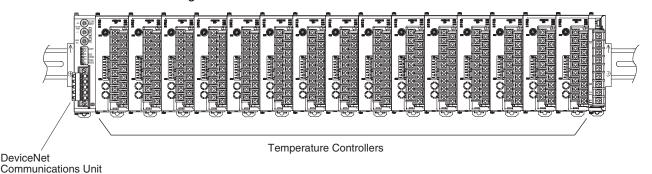
The DeviceNet Communications Unit differentiates each of the connected Temperature Controllers according to communications unit numbers (0 to F: 0 to 15 decimal). The Temperature Controllers can be connected in any order. The communications unit number of each Temperature Controller is set using the rotary switch on the front panel of the Temperature Controller. Always set a unique communications unit number for each Temperature Controller.
