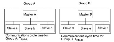
In Networks with two masters, the communications cycle time for the entire Network will be the sum of the communications cycle times for both groups.
