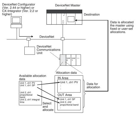
Note: Create the above allocation data using the Configurator's Edit Device Parameters and then download to the DeviceNet Communications Unit.
