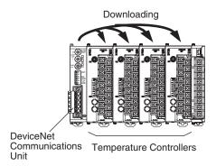
**Note** While downloading, refresh processing of I/O data will stop, and the data immediately before being copied will be held in the IN Area of the DeviceNet Communications Unit. Explicit message communications will stop, so a time-out error may occur.
