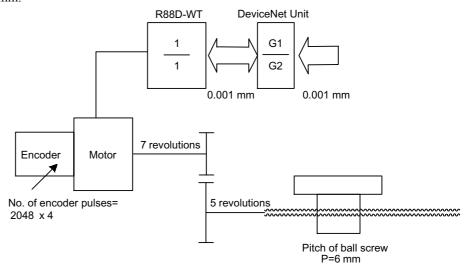
Moving distance of load per revolution (command unit) =  $\frac{\text{Moving distance of load per revolution (mm)}}{\text{command unit (mm)}} = \frac{6 \text{ mm}}{0.001 \text{ mm}} = 6000$
