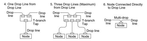
Various combinations of these connections can be used on the same network, as shown in the following diagram.
