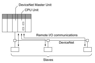
Each slave is allocated words in the I/O Memory in the CPU Unit under which the DeviceNet Master Unit is mounted. There are two methods of allocation: Free and fixed.
