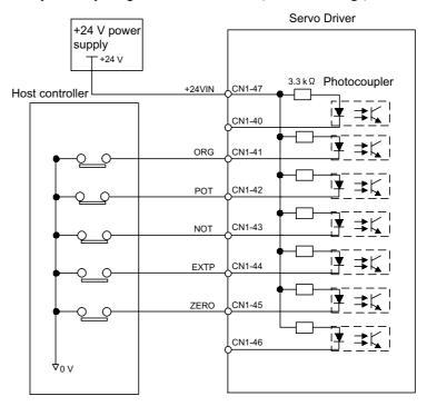
**Note 1.** Provide an external 24-V power supply; the Servo Driver does not have an internal 24-V power supply.
