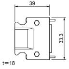
Connector Plug Model 10120-3000VE(20P) (Sumitomo 3M Ltd.) Connector Case Model 10320-52A0-008 (Sumitomo 3M Ltd.)
