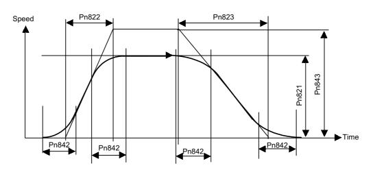
Fig. 5.8 Asymmetric S-curve Acceleration/Deceleration with Constant Acceleration/ Deceleration
