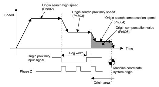
This origin search type returns to the origin using the origin input signal (ZERO signal). The outline of the operation is as follows:
