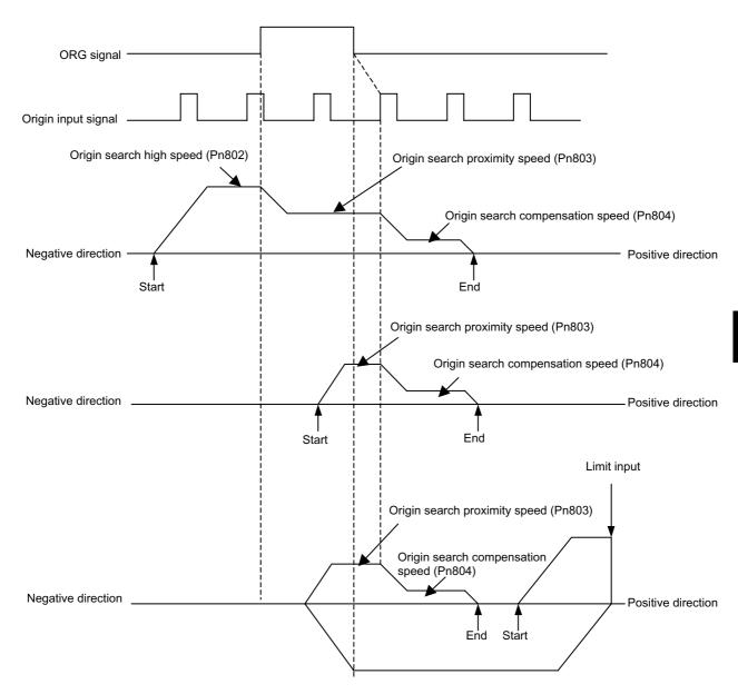
**Note** When the setting for the Origin Compensation Value (Pn805) is small (when the distance is shorter than the distance required for the deceleration from proximity speed), the axis will travel past the origin and then return to it from the other direction.
