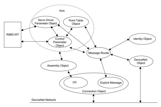
Fig. 10.1 DeviceNet Object Model
