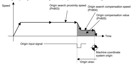
This origin search type returns to the origin using the origin proximity input signal (ORG signal) and the origin input signal (ZERO signal). The outline of the operation is as follows:
