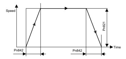
Fig. 5.6 Single-step Linear Acceleration/Deceleration with Constant Acceleration/ Deceleration Time
