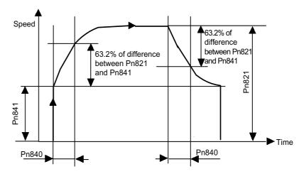
Fig. 5.5 Exponential Acceleration/Deceleration with Bias with Constant Acceleration/ Deceleration Time
