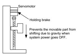
**Note** The brake built into the Servomotor with brakes is a non-excitation brake, which is used only to hold and cannot be used for braking. Use the holding brake only to hold a stopped motor. Brake torque is at least 120% of the rated Servomotor torque.
