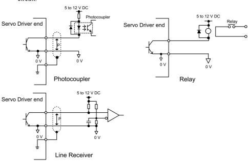
**Note** The maximum allowable voltage and current capacities for open-collector output circuits are as follows:
