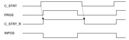
Fig. 6.7 Positioning Command
