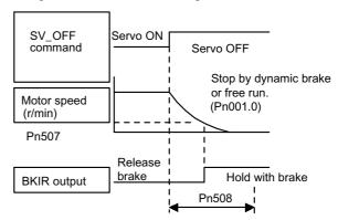
Brake ON timing when the Servomotor stops must be adjusted properly because Servomotor brakes are designed as holding brakes. Adjust the parameter settings while observing equipment operation.
