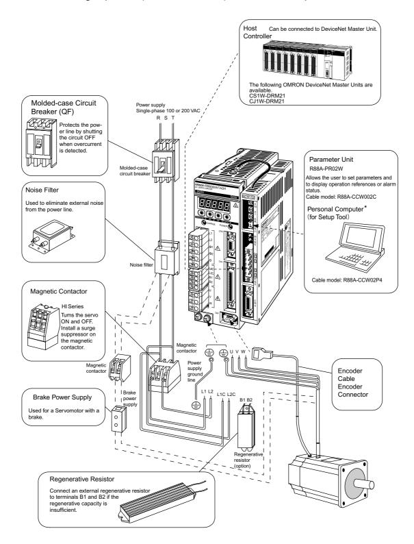
\* A special Setup Tool Cable and the Setup Tool Software (SBCE-001) are required to set and monitor Servo Driver and DeviceNet Unit parameters from a personal computer.
