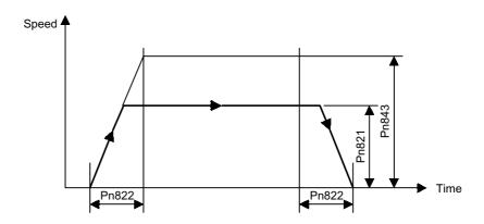
Fig. 5.1 Single-step Linear Acceleration/Deceleration with Constant Acceleration/ Deceleration
