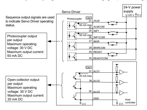
**Note** Provide a separate external 24-V power supply; the Servo Driver does not have an internal 24-V power supply. OMRON recommends using the same type of external power supply as that used for input circuits.
