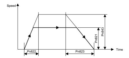
Fig. 5.3 Asymmetric Linear Acceleration/Deceleration with Constant Acceleration/ Deceleration
