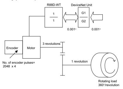
Moving distance of load per revolution (command unit) =  $360^{\circ}/0.001^{\circ} = 36000$
