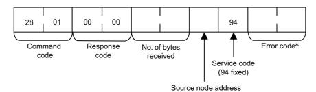
\* For DeviceNet error codes, refer to 10.3.3 Error Codes for Message Communications.
