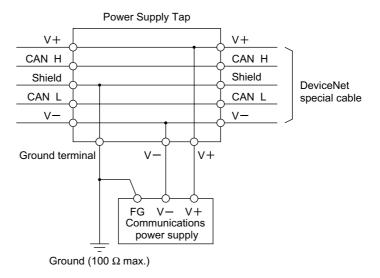
**Note** If more than one communications power supply is connected to the same network, ground only the one nearest the center of the network. Do not connect the shield wire at the other power supplies.
