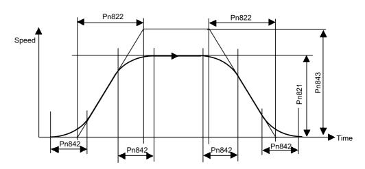
Fig. 5.7 S-curve Acceleration/Deceleration with Constant Acceleration/Deceleration
