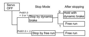
**Note** The dynamic brake electrically applies a brake by using a resistor to consume Servomotor rotation energy. Refer to 8.4.1 Using the Dynamic Brake.
