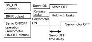
With the standard setting, the servo is turned OFF when the BKIR signal (brake operation) is output. The equipment may move slightly due to gravity depending on equipment configuration and brake characteristics. If this happens, use this parameter to delay servo OFF timing.
