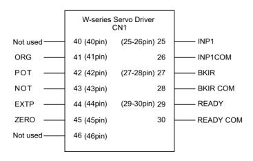
Fig. 8.1 Standard CN1 I/O Signal Settings
