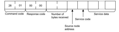
The following example shows the Origin Search High Speed (Object 0x64, instance #1, attribute #12) being read by using the Get\_Attribute\_Single command (code: 0x0e) when the master device node number is 0.
