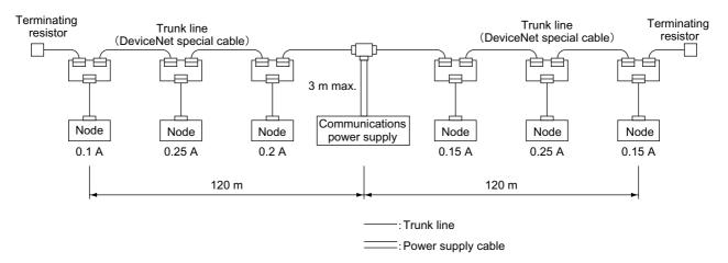
Total power supply length on left = Total power supply length on right = 120 m
