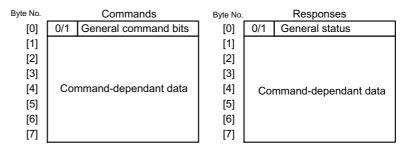
Both the commands and responses are separated into two sections. Byte 0 is a general area and bytes 1 to 7 make up the command-dependant data area. The command-dependant data area depends on the two types of commands, move commands and set/read commands. The type of command is defined by the highest bit of byte 0.
