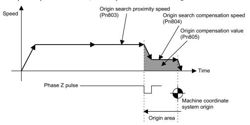
This origin search type returns to the origin using the origin proximity input signal (ORG signal) and the phase Z pulse of the encoder. The axis travels in the reverse direction when the limit input signal of the origin search direction is input. The outline of the operation is the same as Type 0.
