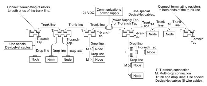
Fig. 4.2 Network Connections
