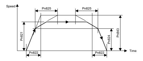
Fig. 5.2 Double-step Linear Acceleration/Deceleration with Constant Acceleration/ Deceleration
