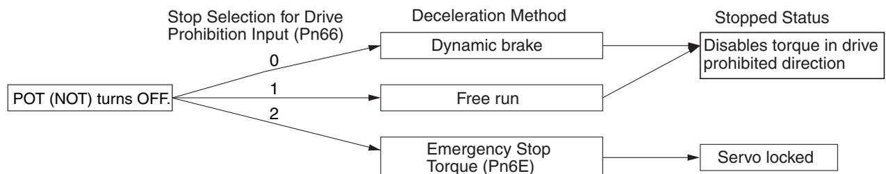
While the Forward Drive Prohibit Input (POT) is OFF, the Servomotor cannot be driven in the forward direction, but it can be driven in the reverse direction. Conversely, while the Reverse Drive Prohibit Input (NOT) is OFF, the Servomotor cannot be driven in the reverse direction, but it can be driven in the forward direction.
