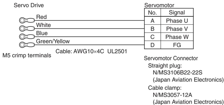
■ Power Cables for Servomotors with Brakes (Standard Cables)
