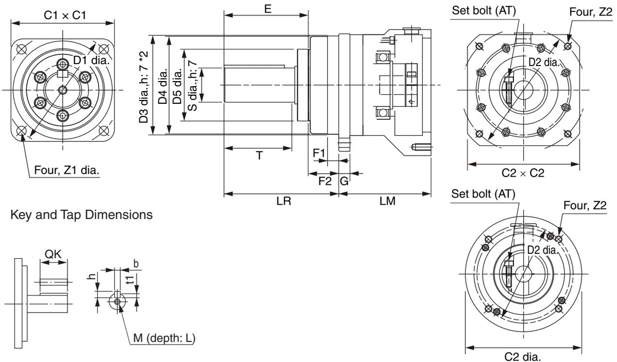
\*2. With the R88G-HPG50□/HPG65□, the height tolerance is 8 mm (D3 dia., h: 8).
