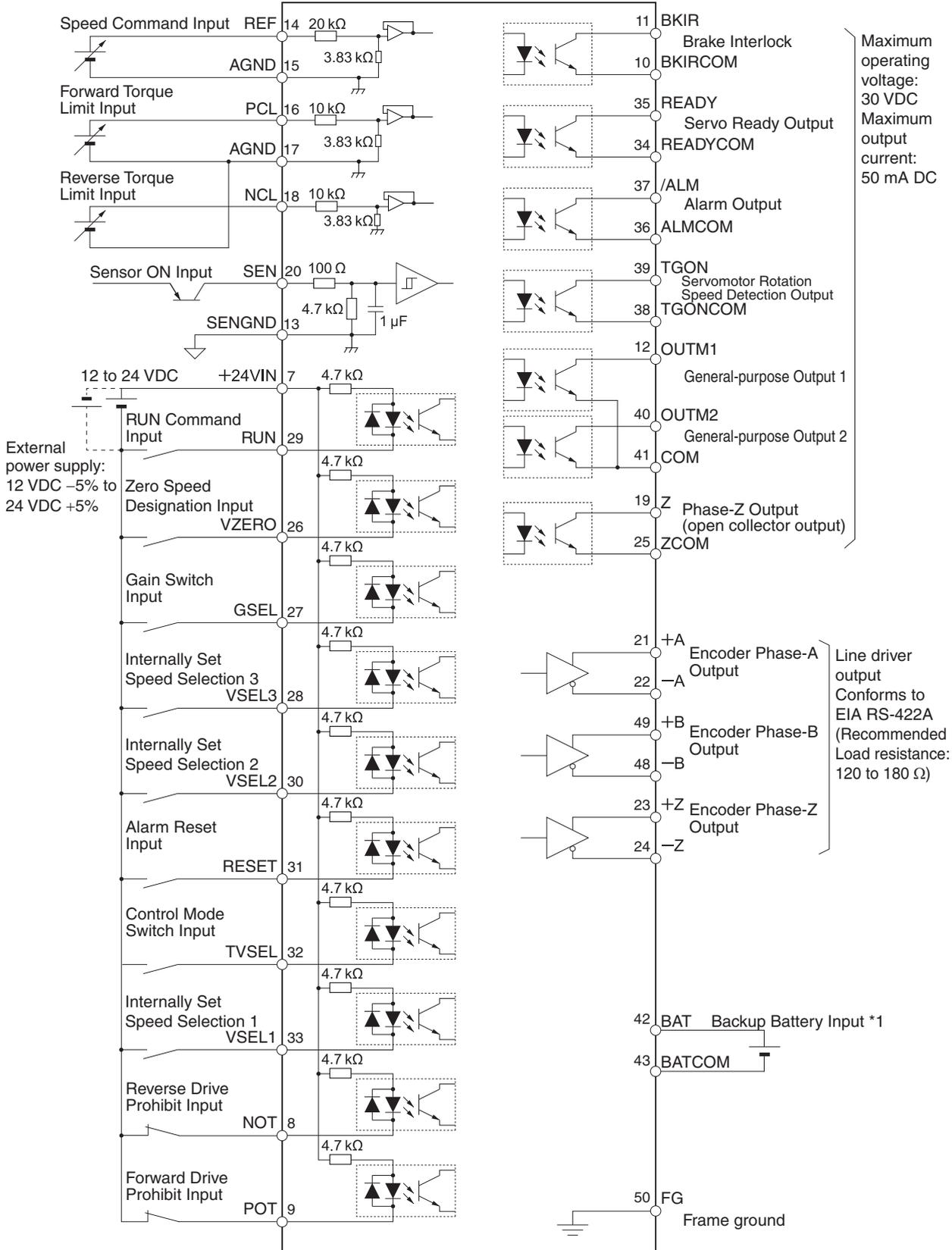
\*1. If a backup battery is connected, a cable with a battery is not required.
