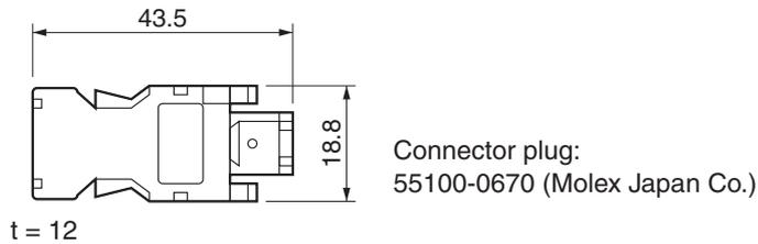
R88A-CNG01R (for Servomotor Connector) **ABS**
