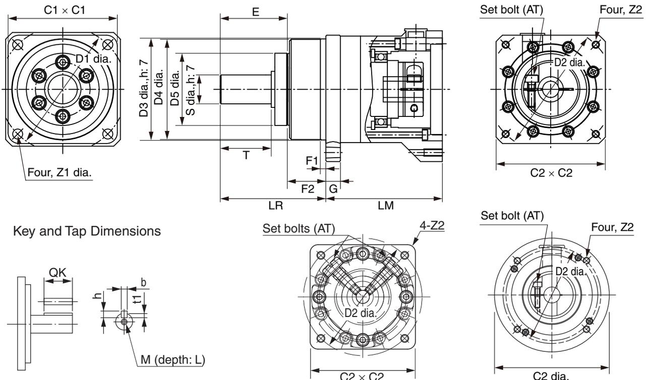
For the R88G-HPG11B Series, two set bolts are positioned at 90° from each other.
