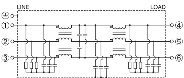
**■ Noise Filter for the Brake Power Supply**
