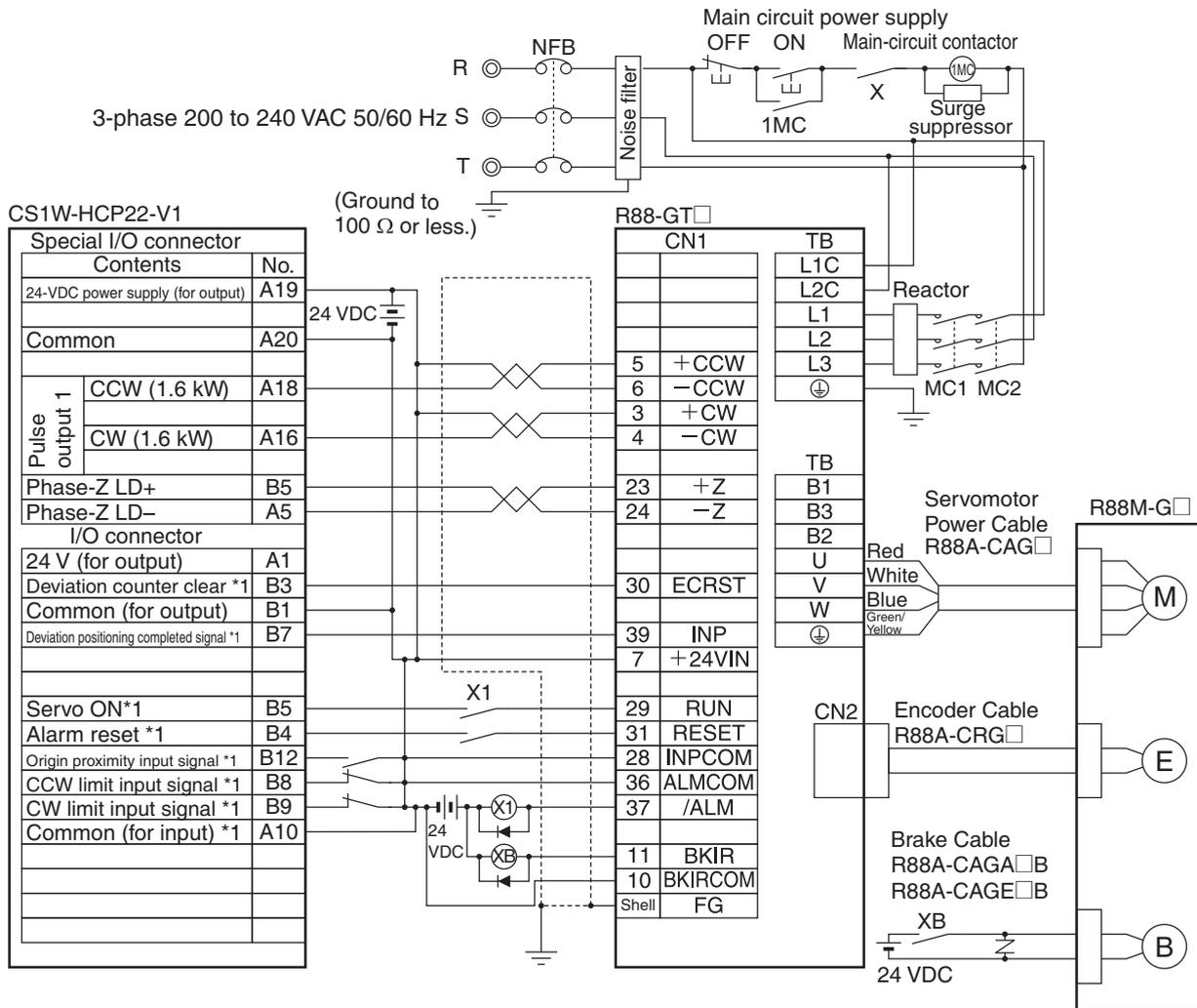
\*1. The I/O bits for the CS1W-HCP22 depend on the memory allocations in the CIO Area. Change the wiring according to the allocations.
