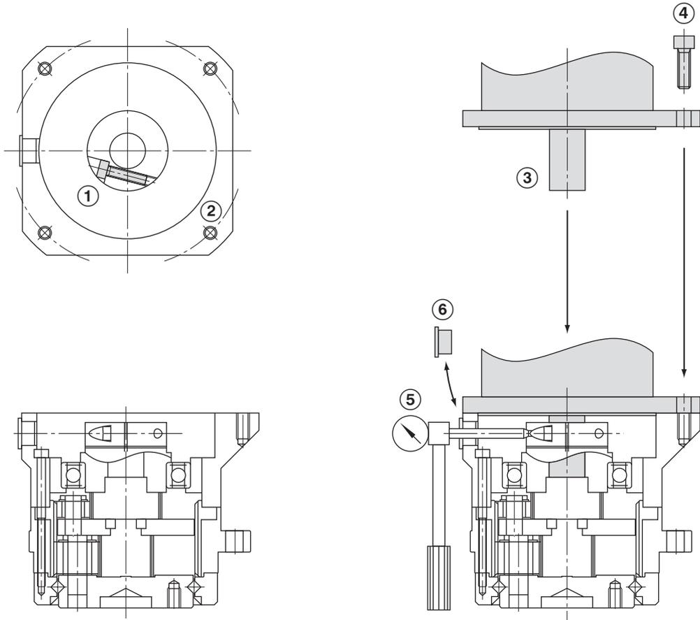
**Installing the Decelerator**
