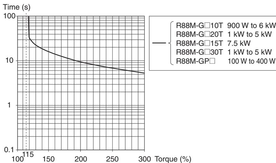
When the torque command = 0, and a constant torque command is continuously applied after three or more times the overload time constant has elapsed, the overload time  $t$  [s] will be:
