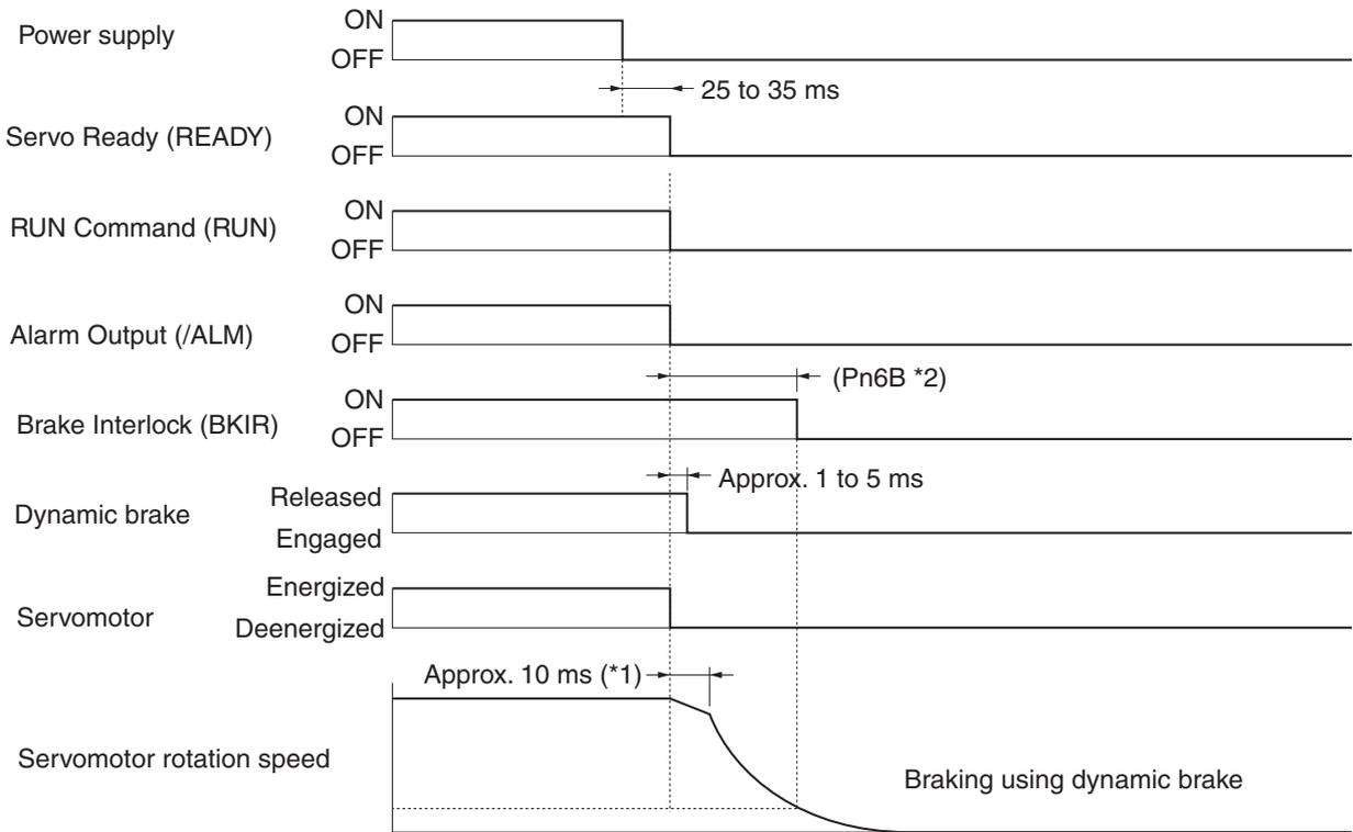
\*1. After the Servomotor is deenergized, it will rotate by inertia for approximately 10 ms until the dynamic brake operates.
