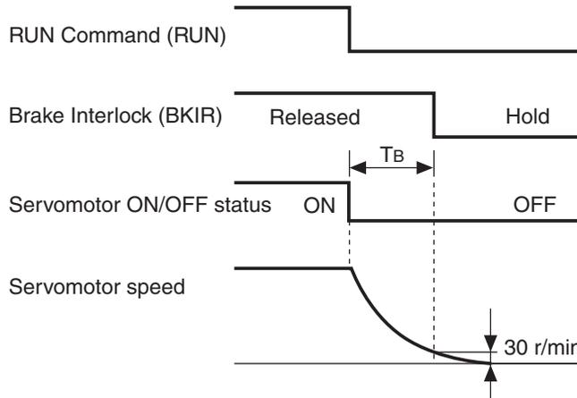
“TB” in the above figure is the brake timing during operation (setting × 2 ms) or the time until the speed of the Servomotor falls to 30 r/min or lower, whichever is shorter.
