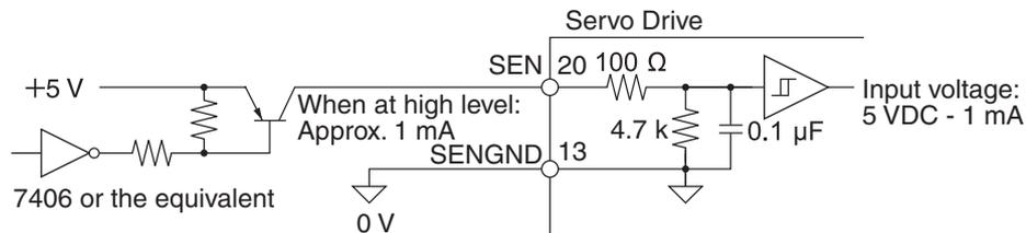
Signal Levels High level: 4 V min.
