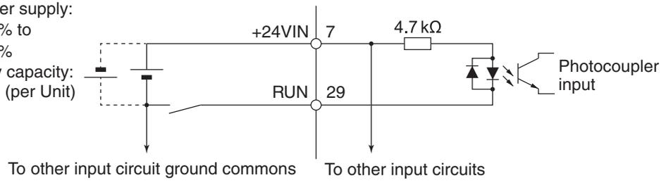
Signal Levels ON level: 10 V min.
