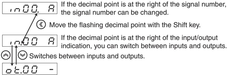
The following procedure can also be used to switch between inputs and outputs.
