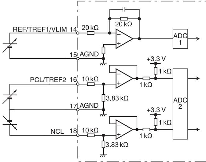
**Precautions for Correct Use** The maximum allowable input voltage is  $\pm 10$  V for each input. The VR must be 2 k $\Omega$  with B characteristics and 1/2 W minimum. R must be 200  $\Omega$  and 1/2 W minimum.
