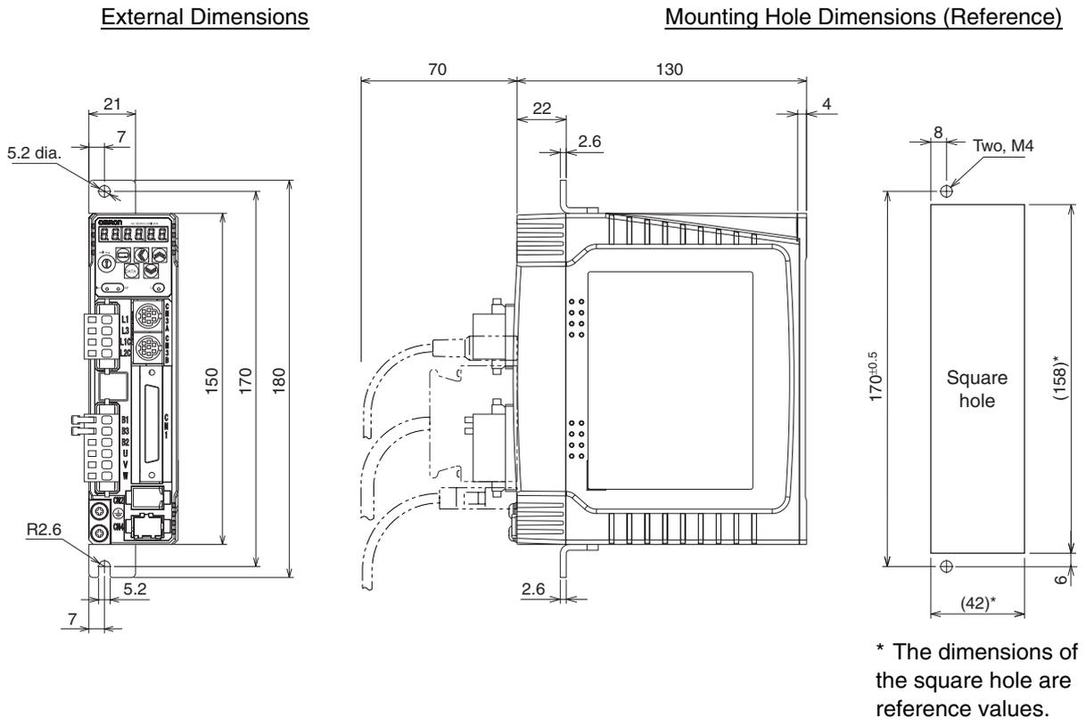
Dimensions for front panel mounting are reference values that provide leeway.
