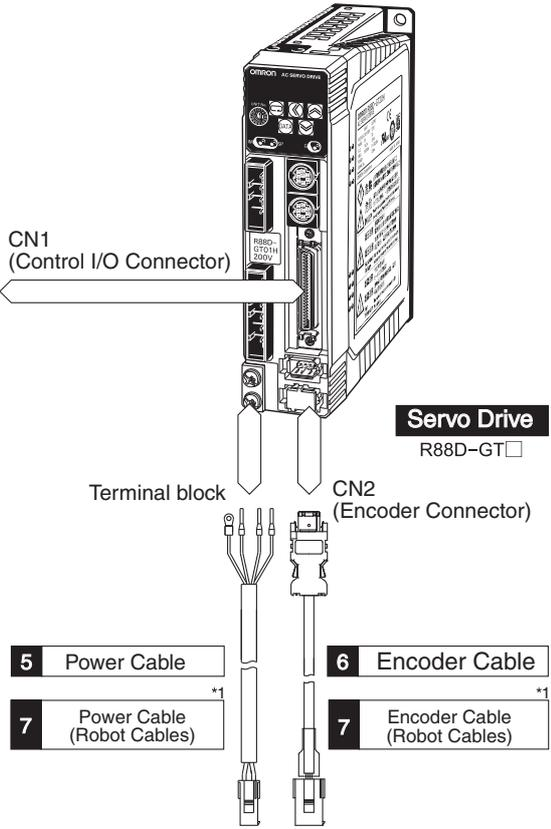
\*1 Use a robot cable when the cable must be flexible.
