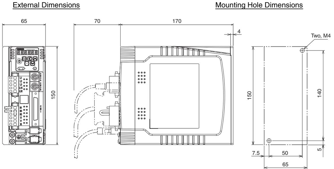
Front Panel Mounting (Using Mounting Brackets)
