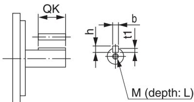
\*2. With the R88G-HPG50□/-HPG65□, the height tolerance is 8 mm (D3 dia., h: 8).
