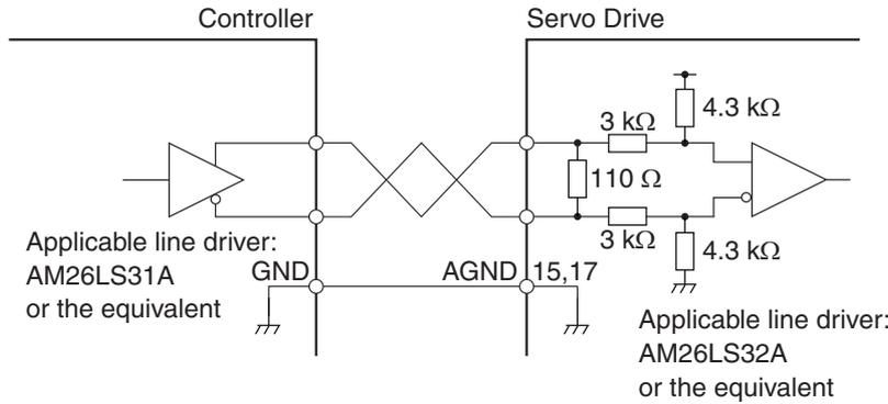
**Precautions for Correct Use** The shielded twisted-pair cable should not exceed 20 m in length.
