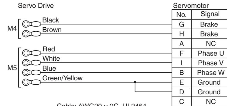
Crimp terminals Cable: AWG20 × 2C UL2464
