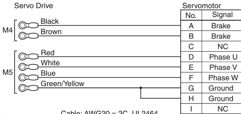
Crimp terminals Cable: AWG20 × 2C UL2464
