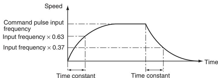
**Note** The time constant will be as follows according to the setting of Pn4C.
