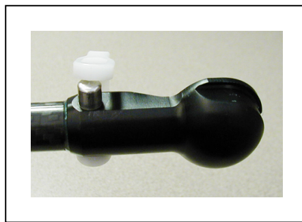
Figure 6-12. Retainer Over Top of Pin
