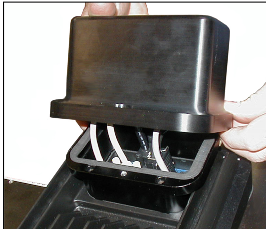
Figure 4-23. Installing Cable Entry Top Cover Assembly
