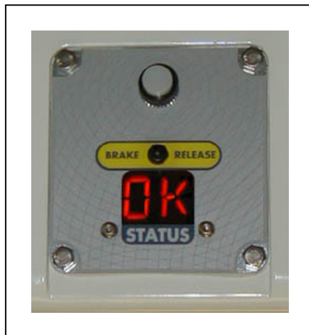
Figure 6-5. iX4-650H/800H Robot Status Panel
