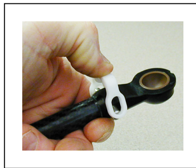
Figure 6-13. Push the retainer Into Position
