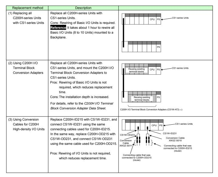
Note 1. Depending on the type of Basic I/O Unit, there may be some restrictions (e.g. change in I/O specifications or wiring) or some models cannot be used.
