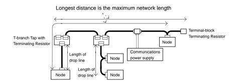
There are two types of cables: Thick cables and thin cables. The thick cables are relatively hard and inflexible, but they protect against signal attenuation and can be used for relatively long communications distances. The thin cables are soft and flexible, but they do not protect as well against signal attenuation and are not suited to long communications distances.
