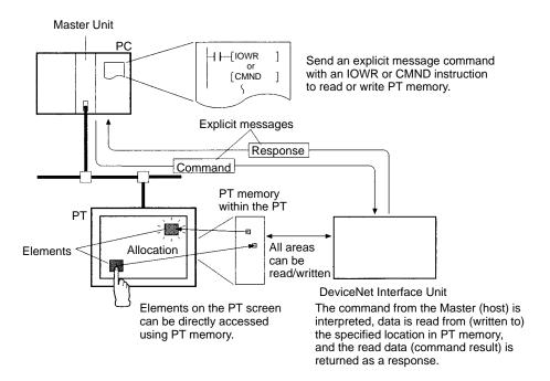
**Reference** 1. Use the EXPLICIT MESSAGE SEND (28 01) FINS command when sending an explicit message from an OMRON Master Unit.
