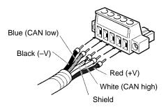
**Note** Be sure the wire set screws are sufficiently loosened before attempting to insert the lines. If these screws are not loose, the lines will enter the gaps in the back of the connector and will not lock properly.
