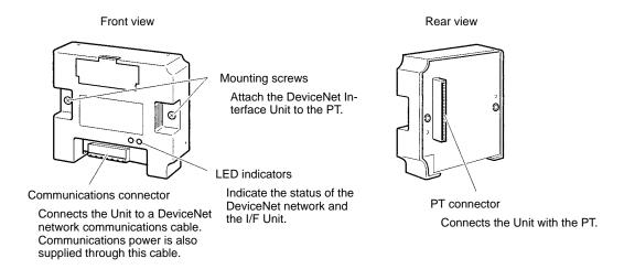
**Note** Inspect the DeviceNet Interface Unit for any damage after removing it from its packaging. Lightly shake the Unit to check whether any parts have broken off inside.
