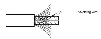
3. Remove the exposed weaving, remove the aluminum tape from the signal and power lines, and strip the covering from the signal and power lines to the proper length for the crimp terminal connectors. Twist together the wires of each of the signal and power lines.
