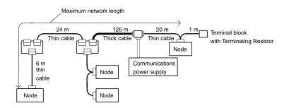
$L_{THICK} + L_{THIN} = 175 \ge 100 \text{ m} \qquad 500 \text{ kbps} \qquad \text{NG}$
