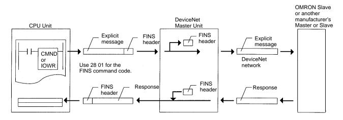
**Reference** When sending an explicit message, specify the DeviceNet Master Unit in the local node as the destination of the FINS command. The final destination Slave (PT) is specified in the command data of the FINS command.
