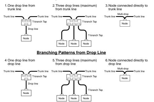
Various combinations of branching patterns can be used on the same network, as shown in the following diagram. Any number of nodes up to 63 can be connected onto a single drop line.
