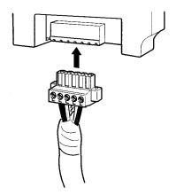
**Note** 1. Before connecting the communications cables, turn OFF the power supply to all PCs, Slaves, and communications power supplies.
