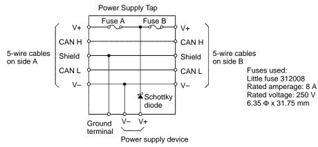
Remove fuse A when disconnecting cables on side A, and fuse B when disconnecting cables on side B.
