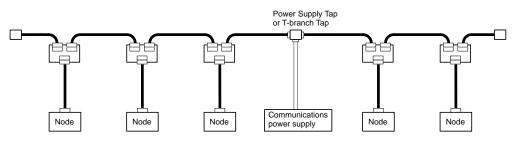
2. Locating the Nodes on One Side of the Power Supply
