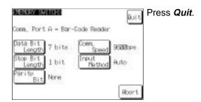
Pressing "Abort" on the communication condition/confirmation method setting screen causes the PT to return to the memory switch setting screen (3/3) without changing the settings. (The previous settings will still be effective).
