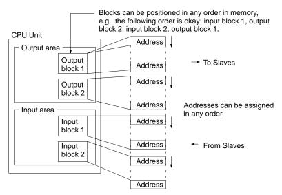
Slaves and blocks can be allocated in any order. The number of words (number of bytes) that are used depends upon the addresses. The minimum is one byte and the maximum is 64 bytes (32 words).
