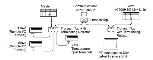
A PT connected to the network through a DeviceNet Interface Unit can perform some of the functions of a control panel, such as switch operations and numeric inputs as well as displaying the system's operating status.
