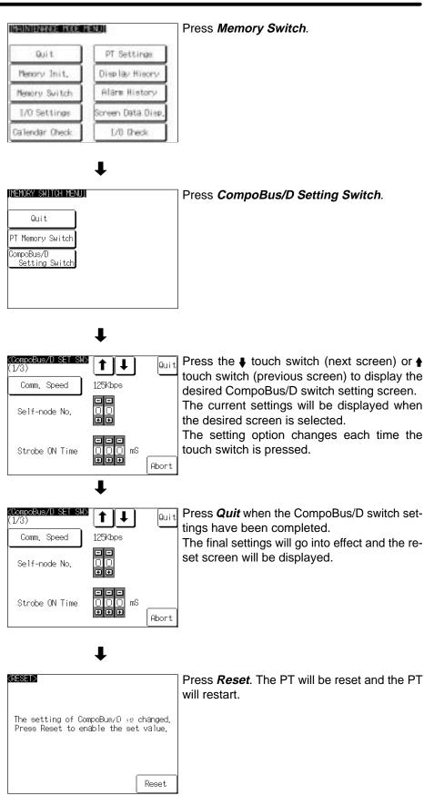
To set other memory switches, select the relevant screen using the ↓ touch switch (next screen) or ↑ touch switch (previous screen) and then make the setting.
