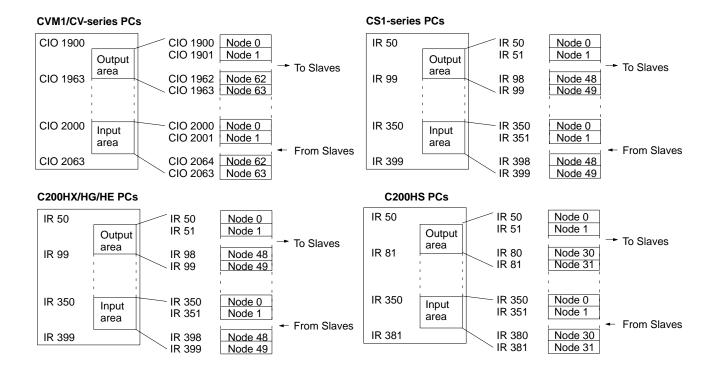
The DeviceNet Interface Unit will occupy the number of words (number of node numbers) set for the input and output areas in the DeviceNet memory switch screen. For example, when the Unit's input area size has been set to 16 words, the output area size has been set to 10 words, and the node number is set to 5, the input area will occupy the words for nodes 5 through 20 and the output area will occupy the words 5 through 14.
