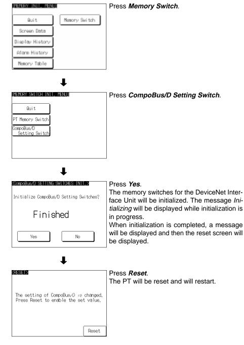
If *No* is pressed in the CompoBus/D setting switch initialization screen, the switch settings will not be initialized and the PT will return to the Memory Init. menu.
