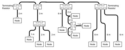
In the configuration example, the length of each drop line is 6 m or less as demanded but the total sum length of all the drop lines is 40 m. Set the baud rate at 250 kbps or 125 kbps because the total maximum length of drop lines at 500 kbps must not exceed 39 m.
