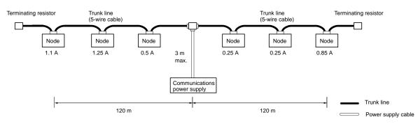
Total power supply length on left = Total power supply length on right = 120 mTotal current consumption on left: 1.1 + 1.25 + 0.5 = 2.85 A
