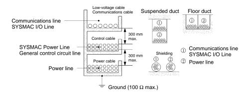
Do not install communications lines and SYSMAC Power Lines onto the control panel on which high-voltage devices are mounted.
