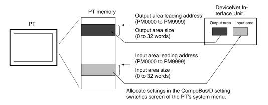
Refer to 5-5 DeviceNet Memory Switch Settings for details on making settings in the CompoBus/D setting switches screen of the PT's system menu.
