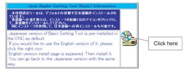
The Basic Setting Tool Installation Page will be displayed. Click the Install Start Button on the left to start installing the English version of the Setting Tool.
