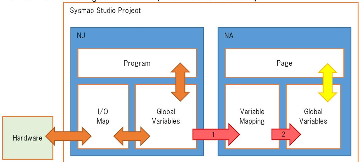
The function is called "variable mapping", and the names of the NA's global variables allocated at this time are specified as "*NJ controller name\_NJ global variable name*". When NA is connected with NJ at 1: N, each NJ is identified by the controller name.
