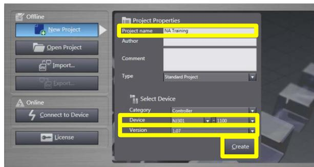
\* Specify the model and version of the NJ to be connected. The versions that are supported for the NA series are 1.01 and later.
