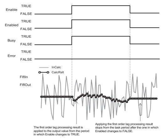
• If the Processing Result (*CalcRslt*) of this function block is nonnumeric or infinity, *Enabled* will change to FALSE. When the Processing Result becomes neither nonnumeric nor infinity, *Enabled* will change to TRUE.
