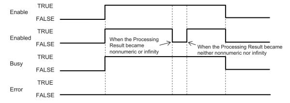
• If an error occurs during function block execution, *Error* will change to TRUE. You can find out the cause of the error by referring to the values output by *ErrorID* (Error Code) and *ErrorIDEx* (Expansion Error Code).
