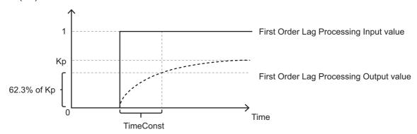
In the above function block, the Laplace operator s is approximated with a backward difference and the following processing is performed.
