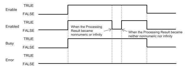
• If an error occurs during function block execution, *Error* will change to TRUE. You can find out the cause of the error by referring to the values output by *ErrorID* (Error Code) and *ErrorIDEx* (Expansion Error Code). When *Enable* to this function block changes to TRUE, *ErrorID* (Error Code) and *ErrorIDEx* (Expansion Error Code) are cleared.
