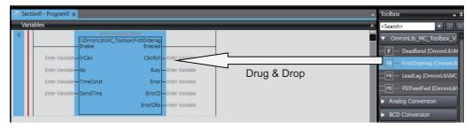
• Right-click the programming editor, select **Insert Function Block** in the menu, and enter the fully qualified name (\name of namespace\name of function block).
