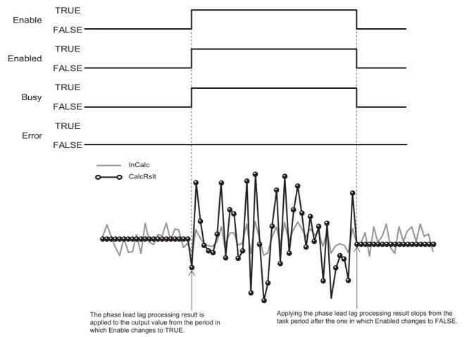
If the Processing Result (CalcRsIt) of this function block is nonnumeric or infinity, Enabled will change to FALSE. When the Processing Result becomes neither nonnumeric nor infinity, Enabled will change to TRUE.
