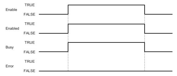
• If the Processing Result (*CalcRslt*) of this function block is nonnumeric or infinity, *Enabled* will change to FALSE. When the Processing Result becomes neither nonnumeric nor infinity, *Enabled* will change to TRUE.
