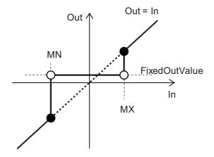
The input value (In) is converted as given in the following table for the Upper Limit (MX), the Lower Limit (MN), and the Fixed Output Value (FixedOutValue).
