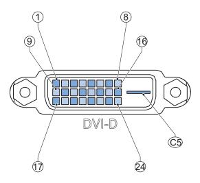
The pin layout represents the DVI connector on the Industrial Panel PC. Pin numbers increase from left to right for every row.
