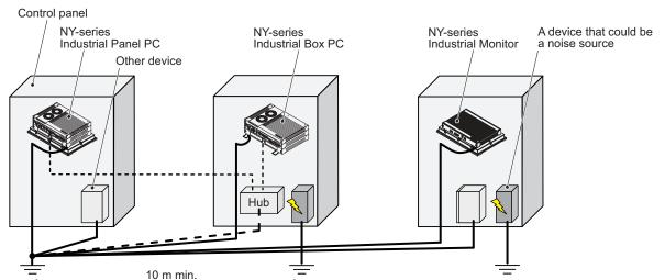
b. Connecting devices and noise sources to a common earth electrode
