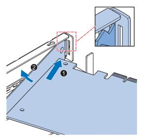
Ensure to insert the PCIe Card in the correct opening.
