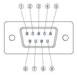
The pin layout represents the RS-232C connector on the Panel PC.
