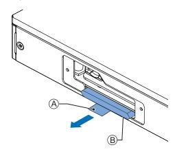
4 Insert the replacement CFast Card (A) into the slot of the Panel PC.
