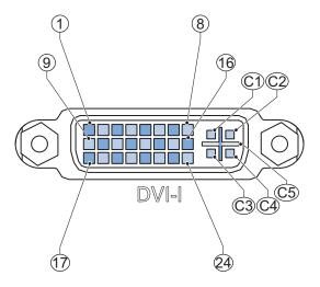
The pin layout represents the DVI-I connector on the Industrial Panel PC. Pin numbers increase from left to right for every row.
