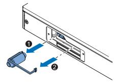
**4** Connect the new battery to the battery connector **2** and then insert the new battery **1** in the battery holder.
