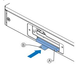
Fold the plastic Pull Tab (B) up so it stays inside the slot area.
