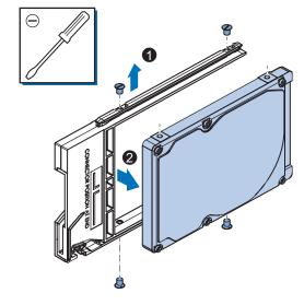
7 Align the connectors of the replacement drive as shown on the bracket. Then insert the replacement drive in the bracket and insert the 4 mounting screws Tighten these screws with a torque of 0.35 N·m.
