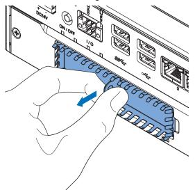
**4** Rotate **1** and then remove **2** the break out part from the drive bracket.
