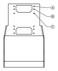
**3** Tighten the 4 screws with a torque between 2.5 and 3.0 N m with a hexagon tool.
