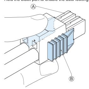
Do not push the orange sliders <sup>(B)</sup> in the direction of the Panel PC because this will unlock the connector.
