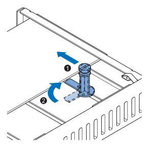
Ensure the Card Support contacts the PCIe Card with the small groove so that there is support below and above the PCIe Card.
