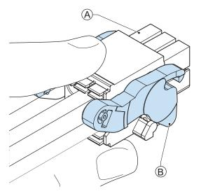
Do not tilt the orange levers (B) because this will unlock the connector.
