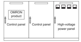
**Example of Poor Equipment Arrangement**
