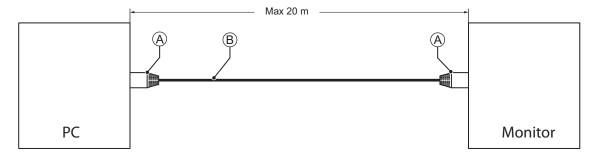
The following table lists the recommended cables and connectors for the NY Monitor Link cable applications up to 20 m.
