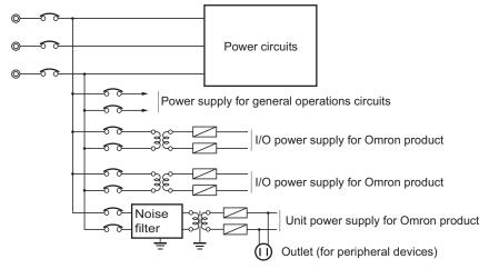
Power Supply System Diagram
