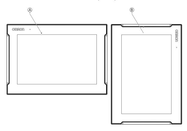
Do not install the Industrial Panel PC in any of the following orientations.
