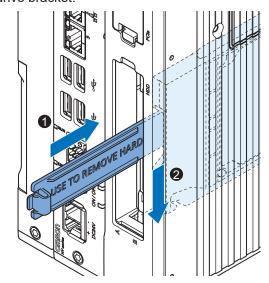
**5** Remove the drive bracket from the Panel PC using the drive cover.
