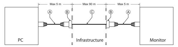
The following table lists the recommended cables and materials for the NY Monitor Link cable applications up to 100 m.
