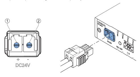
The pin layout represents the power connector on the Panel PC.
