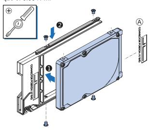
6 Insert the bracket with the drive in the correct bay.
