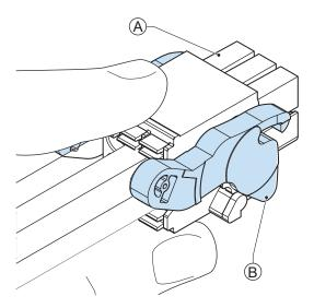
Tilting both levers <sup>®</sup> will release the I/O connector <sup>®</sup> from the Panel PC.
