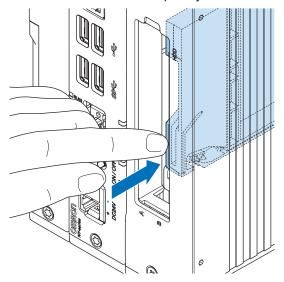
The drive bracket will lock into place when it is fully inserted.
