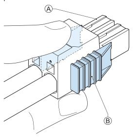
Pushing both orange sliders <sup>(B)</sup> towards the end of the connector <sup>(A)</sup> will release the lock when removing the connector.
