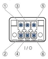
The pin layout represents the I/O connector on the Panel PC.
