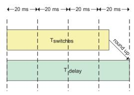
Fig. 2-11 Zone Delay configuration.
