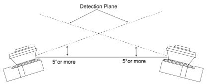
Fig. 4-2 Offset Scanning Level by Tilting
