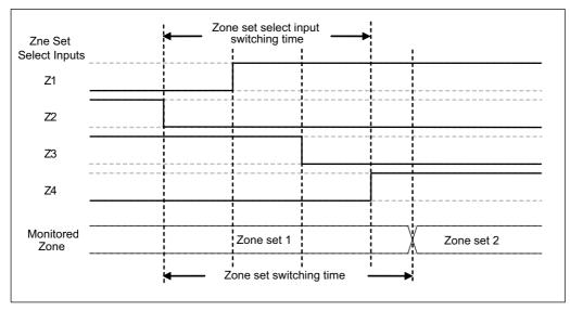
Fig. 2-9 Zone Switching example
