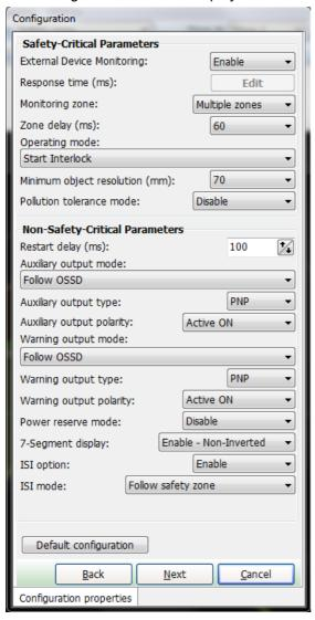
Fig. 3-18 New Configuration Parameters for OS32C-xxx and OS32C-xxx-4M
