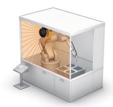
Fig. 1-5 Vertical Guarding Installation
