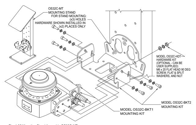
Fig. 4-35 Mounting Stand Assembly OS32C-MT
