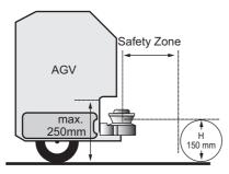
Fig. 4-12 Installation on Automated Guided Vehicle
