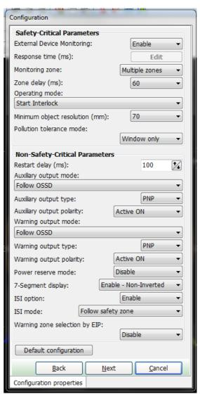
Fig.3-18b New Configuration Parameters for OS32C-xxx-DM and OS32C-xxx-DM-4M
