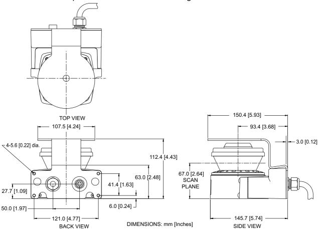
Fig. 4-20 Dimensional drawing of OS32C with Top Guard Kit OS32C-BKT4
