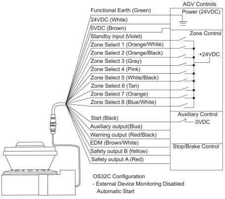
Fig. 5-4 Connecting to AGV Controls
