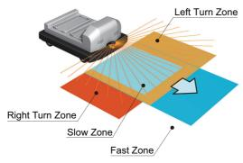
Fig. 1-9 Automated Guided Vehicles, Multiple Zones (AGV)
