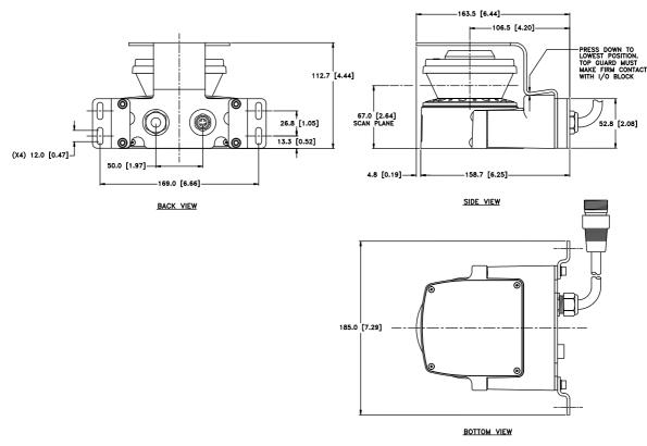
Fig. 4-24 Dimensional drawing of OS32C with OS32C-BKT3 and OS32C-BKT4
