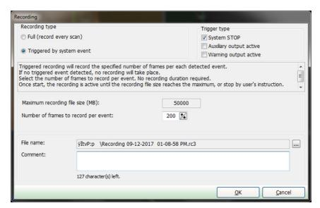
Fig. 3-80 Event Triggered Recording
