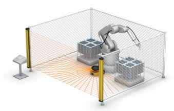
Fig. 1-4 Internal Robot Cell Guarding
