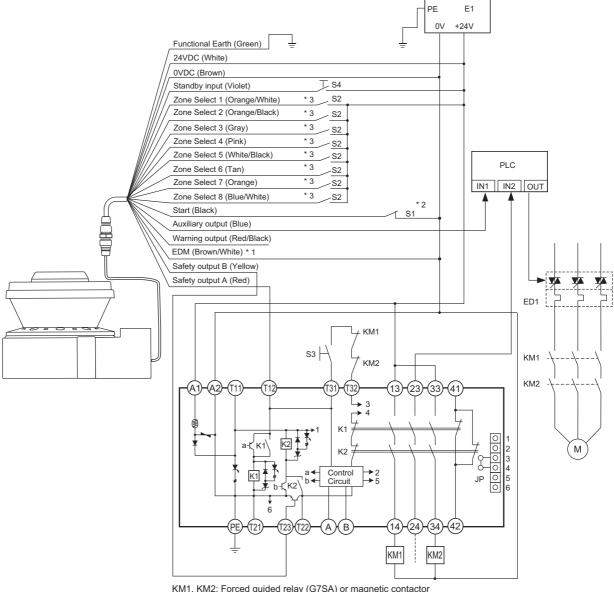
KM1, KM2: Forced guided relay (G7SA) or magnetic contactor
