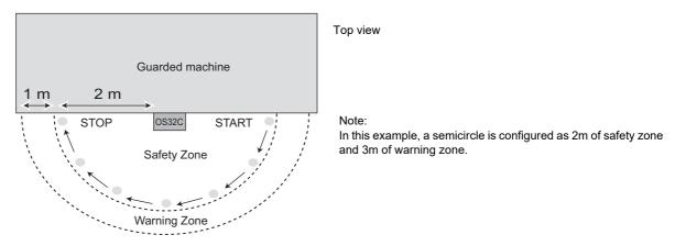
Fig. 6-1 Testing a Horizontal Safety Zone
