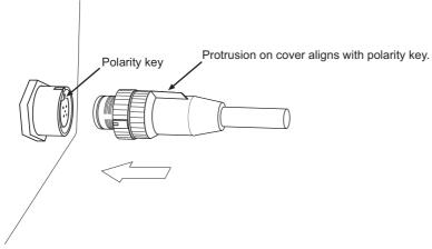
Fig. 4-38 Aligning to polarity key
