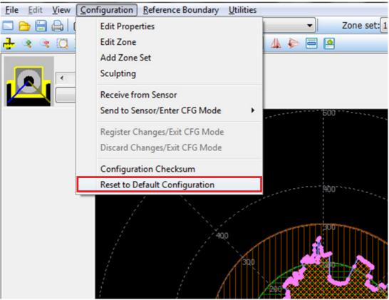
Fig. 3-93 Reset to Default Configuration
