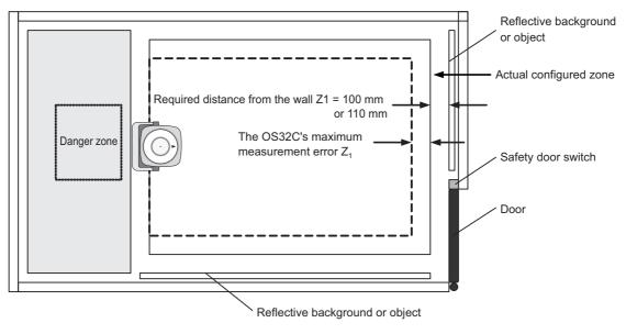
Fig. 7-5 Installing Door on Entrance
