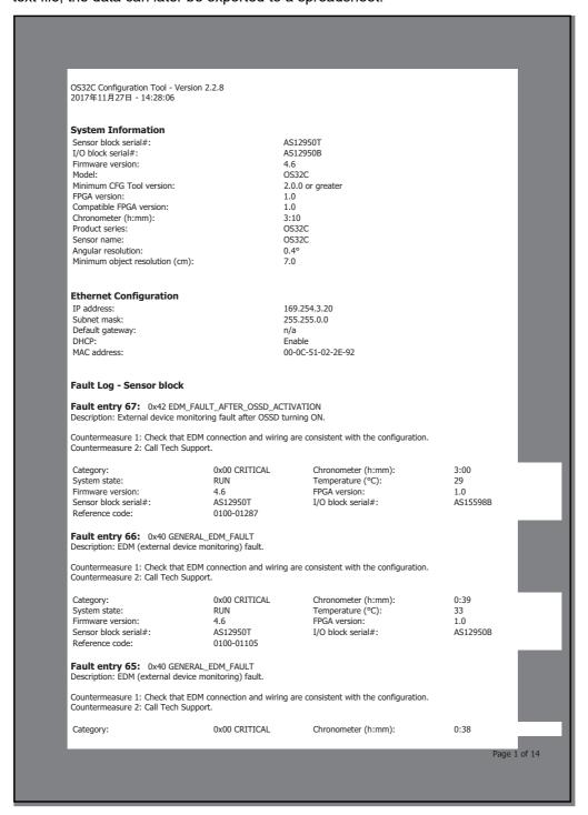
Fig. 3-84 Fault Log
