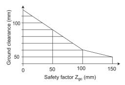
Fig. 4-16 Safety Factor for Low Ground Clearance
