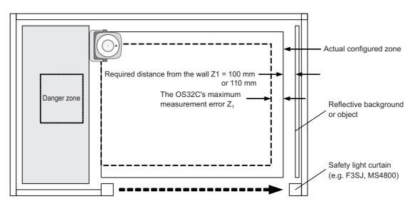
Fig. 7-4 Installing Safety Light Curtain on Entra7-4nce
