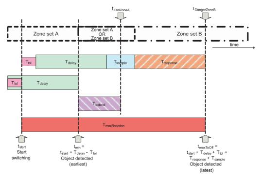
Fig. 2-13 Object detection in Zone set B.
