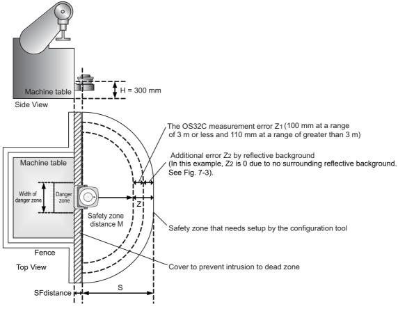
Fig. 4-7 Installation on a Machine
