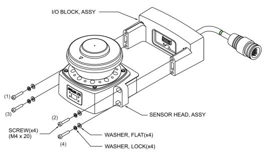
Fig. 7-9 Sensor Block Replacement
