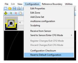
Fig. 7-10 Reset to Default Configuration
