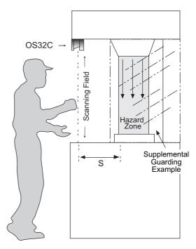
Fig. 4-11 Hand Detection Protection
