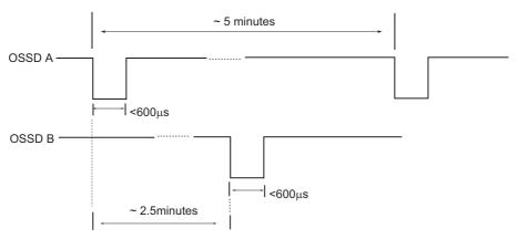
Fig. 2-1 OSSD Test Pulses
