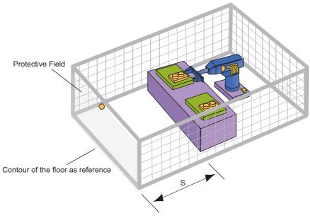
Fig. 4-10 Perpendicular Approach Installation
