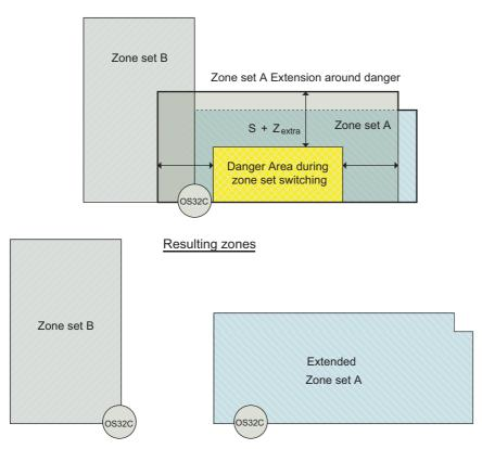
Fig. 7-20 Zone set A extension on limited danger area (example 1).
