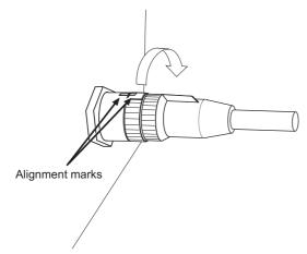
Fig. 4-40 Aligning the XS5 Plug
