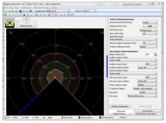
Fig. 3-1 OS32C Configuration Tool
