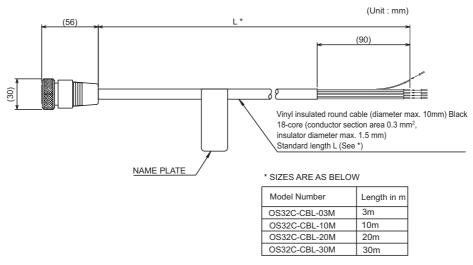
Fig. 4-36 External dimensional drawing of power cable
