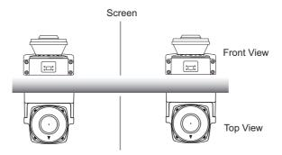
Fig. 4-4 Separation using a screen
