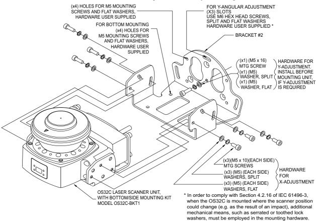
Fig. 4-31 Assembly drawing of OS32C with OS32C-BKT1 and OS32-BKT2
