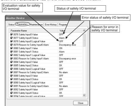
2. Click the **Parameters** Tab in the Monitor Device Window.
