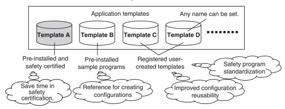
**IMPORTANT** Even when using a safety-certified application template, confirm that the safety functions are working correctly in the environment where they are to be used before beginning system operation.
