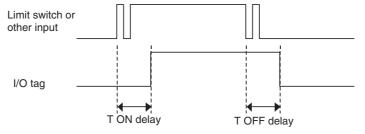
**IMPORTANT** Add both the input ON delay and input OFF delay to the I/O response performance. For further details, refer to 3-2 Reaction Time.
