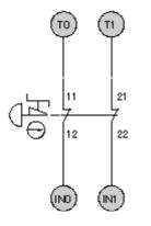
If detecting short-circuits between input wiring is required.
