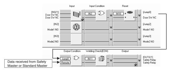
Safety Input Logic Parameter Setting Operations
