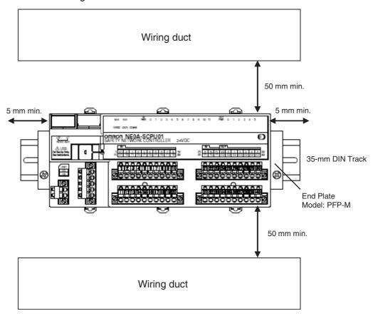
**Note** The NE0A-series Controller can be mounted only to DIN Track. Do not screw the Controller to the control panel.
