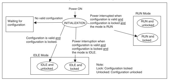
The following diagram shows mode changes for RUN Mode, IDLE Mode, and CONFIGURING Mode.
