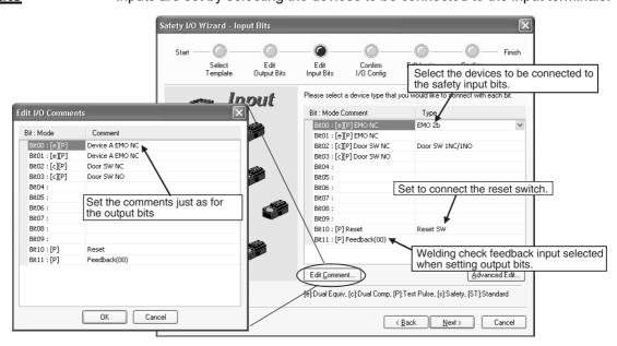
**Note** The leftmost two bits (bit 10: IN10, bit 11: IN11) can be selected only for reset switches or welding checks.
