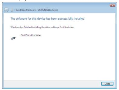
8. The Found New Hardware Dialog Box will be displayed again, because Network Configurator version 3.3 or higher requires two drivers. Perform the installation using the procedure in steps 2 to 7.
