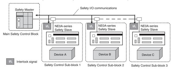
NE0A-series Controllers can be used to construct this type of system, and the configuration and setup can be executed individually for each safety control block.
