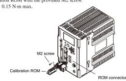
efore pushing in or pulling out the calibration ROM, be sure to turn off the power of the Sensor Controller. Otherwise, a failure might be caused
